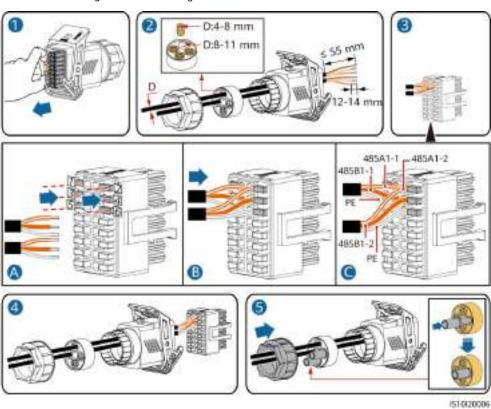
2. Connect the signal cable connector to the communication port.
