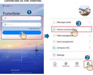
2. Connect to the solar inverter WLAN and log in as **installer** to access the device commissioning screen.
