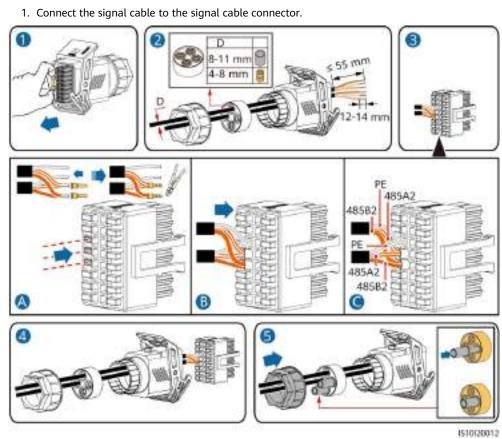
2. Connect the signal cable connector to the Communication port.
